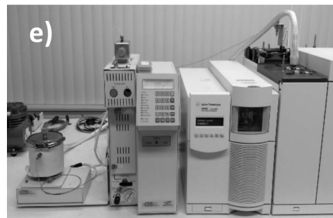
Sample material joining research equipment at Oakland University (a. Autoclave bonding, b. Ultrasonically-controlled joining, c. Surface profiler, d. DMA, e. GCMS Gas Chromatography – Mass Spectrometry system)
